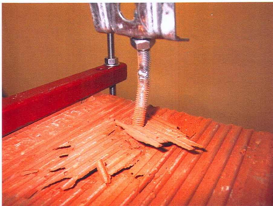
Method of rupturing the threaded rod and hollow brick.
